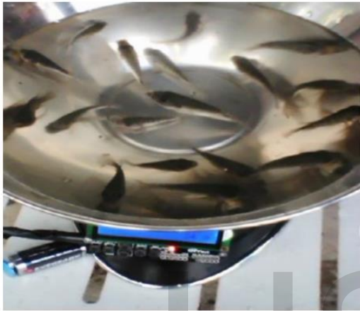
Figure 6. Counting fry using Constructed counter showing fish fry freely moving in the fry holder
